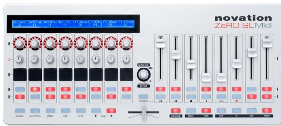
12 pav. Novation ZeRO SL Mk2 MIDI valdiklis (en.audiofanzine.com, 2020)
