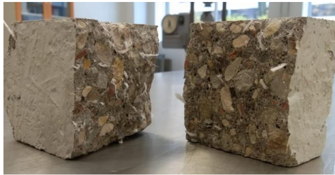
Fig. 4.2. 9. Fibers after breakage (10UCR)
