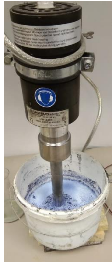
Fig. 2. 5. Crumb rubber dispersed in SBR latex under the ultrasonic dispersion method
