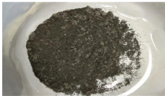
Fig. 2. 3. Unsieved fibrous crumb rubber ( >0.315\text{mm} )
