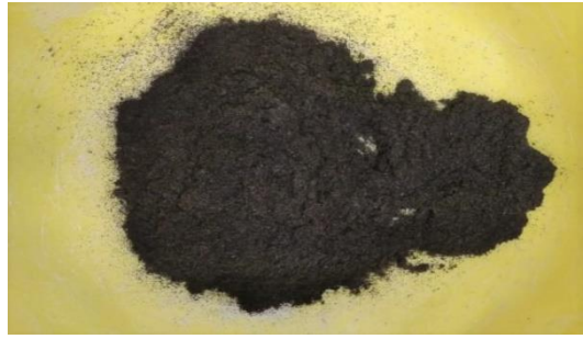
Fig. 2. 4. Sieved fibrous crumb rubber (<0.315mm)
