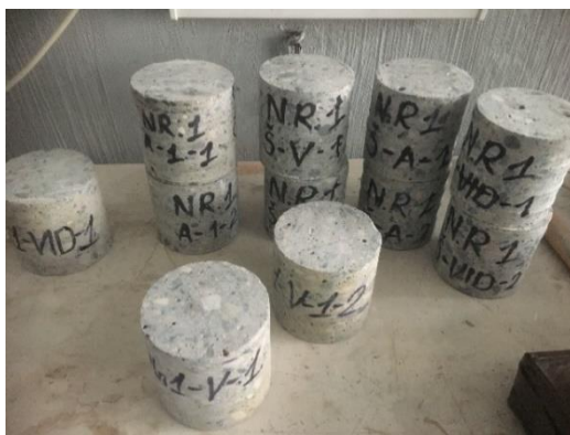
30 pav. Cilindro formos kernos 100x100mm
