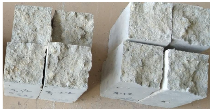
Fig. 30. Macroscopic structure of samples with treated wood fibres and zeolite (hydrosodalite)
