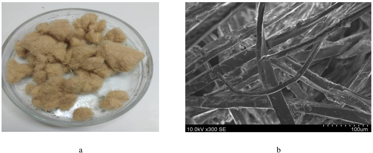
Fig. 10. Structure of wood fibres. Here a - macrostructure of fibres; b - microstructure of fibres
