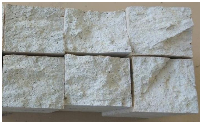
Fig. 23. Macroscopic structure of samples with treated wood fibres and zeolitic waste
