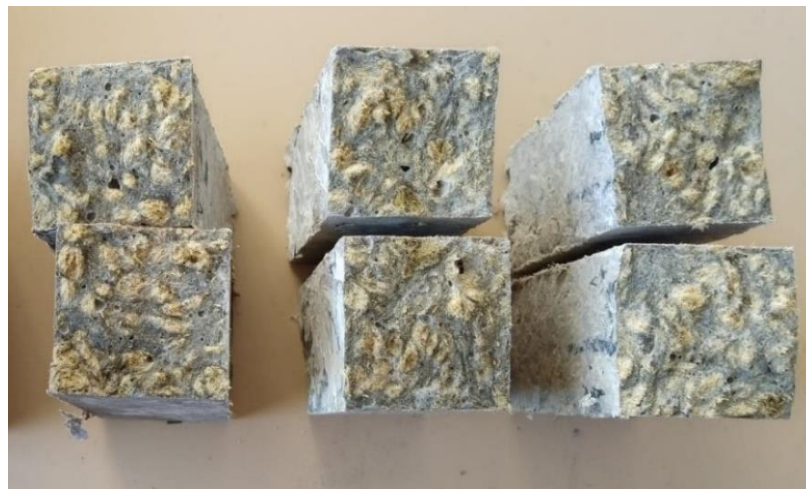
Fig. 19. Macroscopic structure of samples with untreated wood fibres and zeolitic waste
