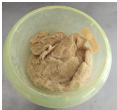
Fig. 17. Treated wood fibres after ultrasonic dispersion
