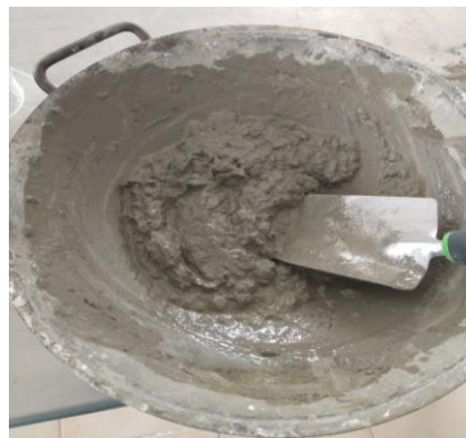
Fig. 16. Homogeneous wood-fibres cement composite paste
