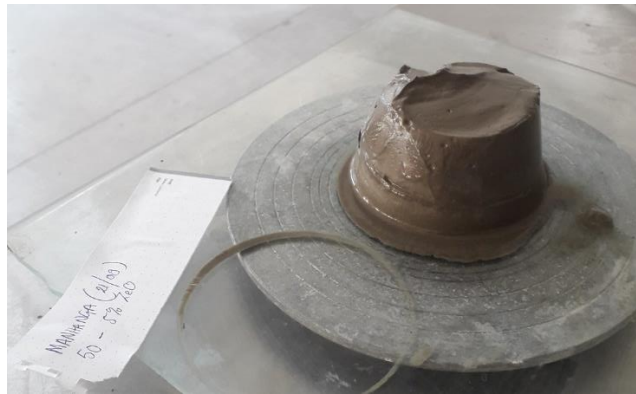
Fig. 14. Photo showing slump of cement paste containing 5% zeolite by mass
