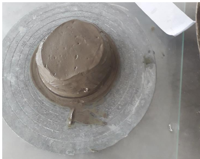
Fig. 15. Photo showing slump of cement paste containing 10% zeolite by mass
