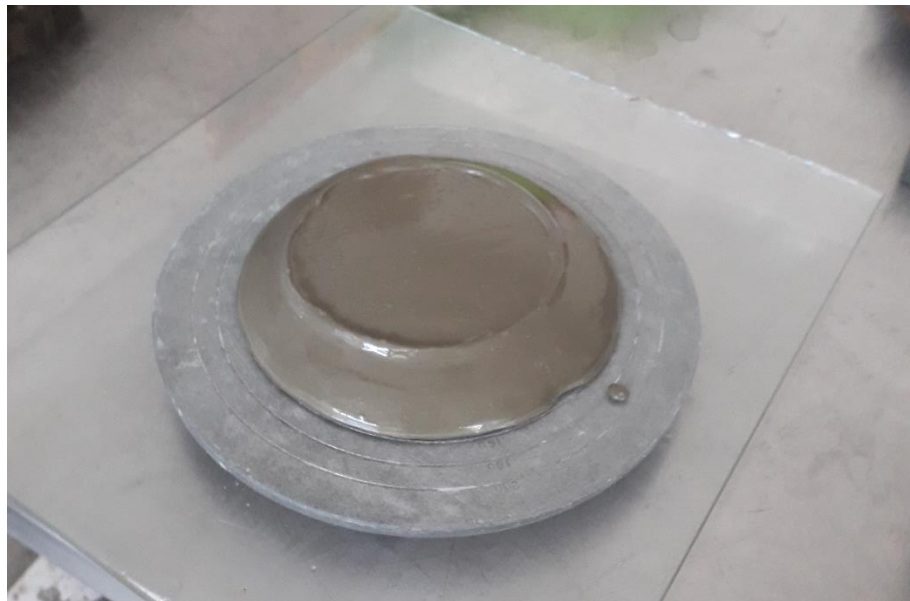
Fig. 13. Photo showing slump of cement paste with no zeolite
