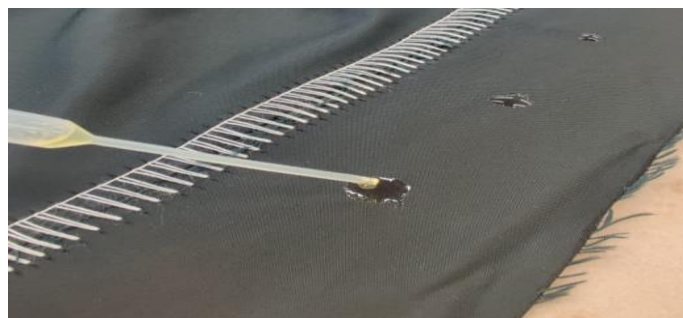
Fig. 17. Dropping oil to make stains
