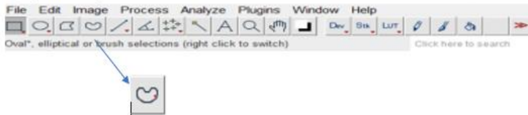
Fig. 28. A tool to measure irregular defects
