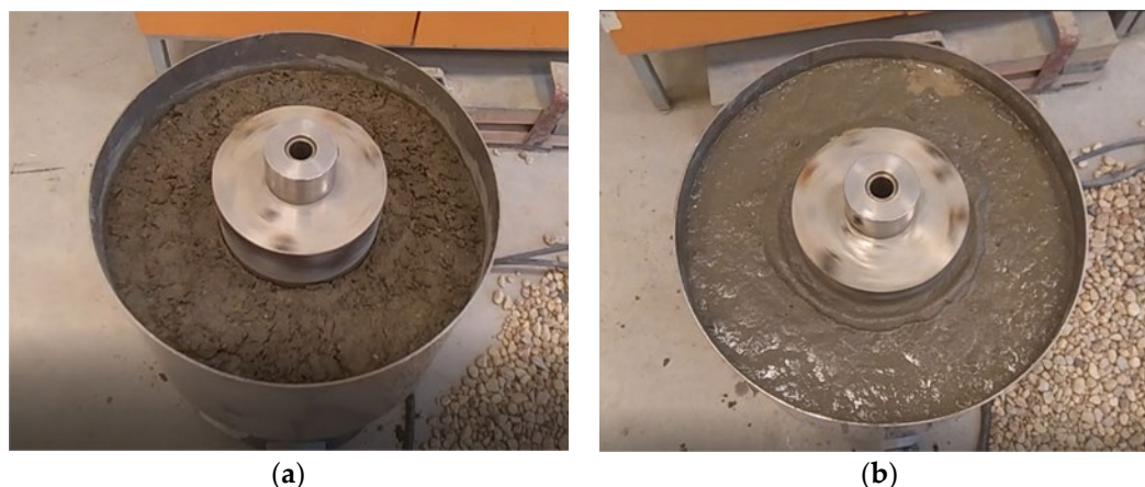
Figure 4. The scenarios observed during testing: (a) partial shearing of concrete, (b) shearing was localised at the concrete steel interface.
