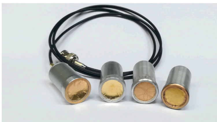
Figure 2. Picture of transducer prototypes, from left to right: HS03 focused (radius of curvature: 22 mm), HS03 focused (radius of curvature: 35 mm), HS06 flat, HS03 flat.
