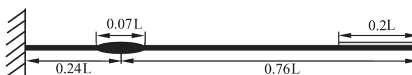
Figure 7. Optimized MFC-magnet energy harvester mechanical structure.
