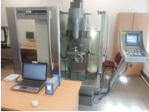
Fig. 2 Experimental setup of the friction drilling experiment
