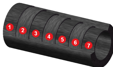
Fig. 3 Layers structure of experimental tube: 1, 3, 5 and 7 are longitudinal layers; 2, 4 and 6 - transverse layers
