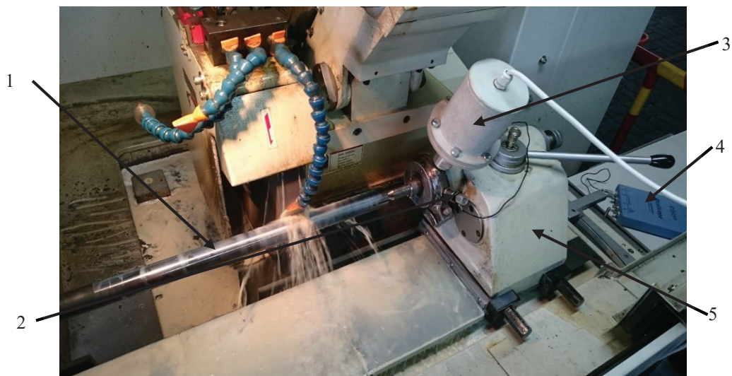
Fig. 60. Experimental setup of ultrasonic-assisted grinding. 1 – Workpiece 1 (steel bar); 2 – accelerometer ( KD35 ); 3 – piezoelectric transducer; 4 – PicoScope (3424); 5 – tailstock of a cylindrical grinding machine ( Supertec G32P-100NC )
