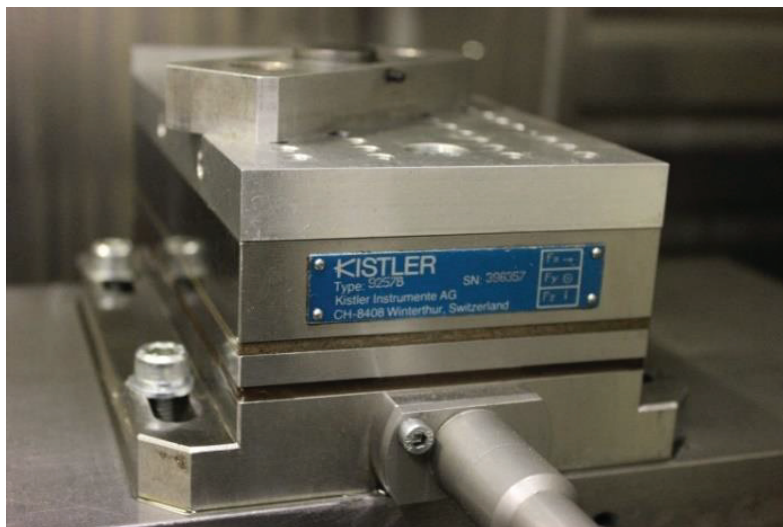
Fig. 48. Kistler 3 channel 9257B force sensor
