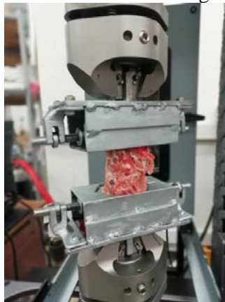
Fig. 3.13. Spinal functional unit placed in holders
