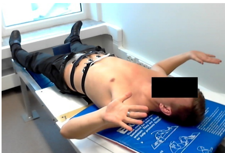
Fig. 4.5. Subject performing lateral bending moves on spinal actuator with sensors placed on the skin above the muscles
