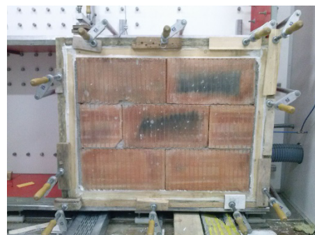
Fig. 3. Specimen of ceramic blocks masonry filled with horizontal joints mounted into air permeability measuring device.
