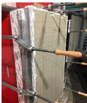
Fig. 4. Wall sample installed into test device: drilled wood fiber cement board + insulation in wooden frame.
