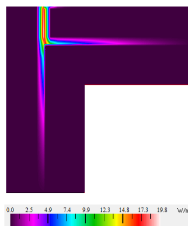
Fig 5. The intensity of heat flow through the wall corner insulated with aluminium foil faced PIR, without PU glue
