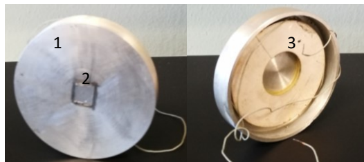
Fig. 4. 4 Disc-shaped control platform (1) with a micro optical element (2) and an active piezoelectric element (3)
