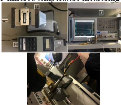
Fig. 3. 9 BGI mark – 10 force / torque gauge (1) force gauge controller (2), 6500B series of Precision Impedance Analyzers (3), Sonotrode (4) Testo 845 Infrared temperature measuring instrument (5)
