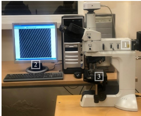
Fig. 3. 24 Optical microscope: Optical microscope connected to PC (1), PC for reading (2), Specimen (3)
