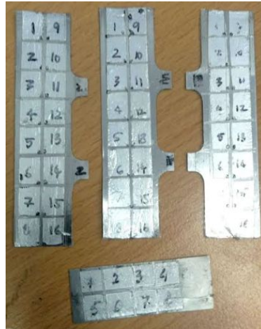
Fig 34. The aluminum foil cantilevers used to measure quality of glue
