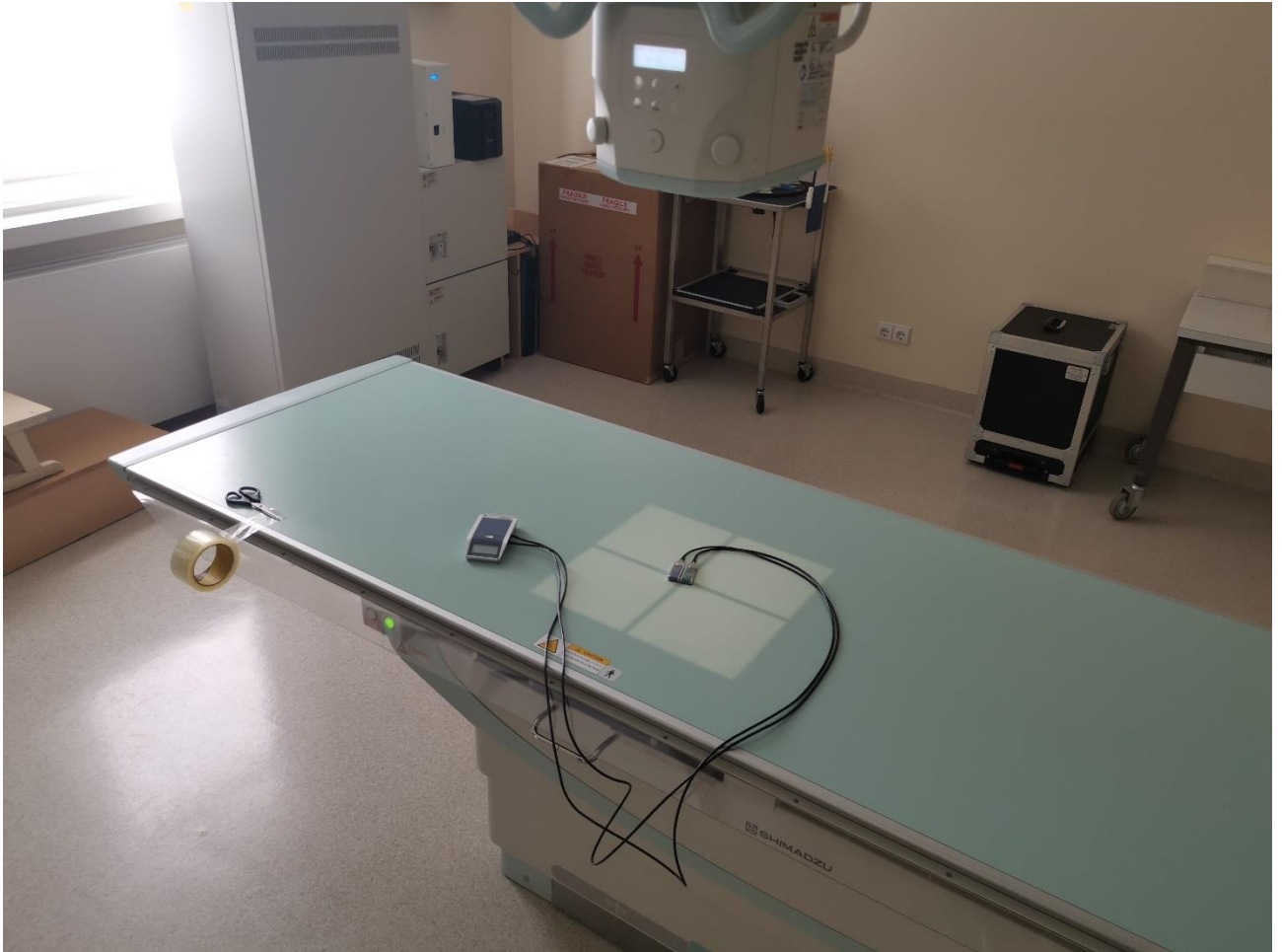
Fig. 2 X-ray machine radiation output measurement set up
