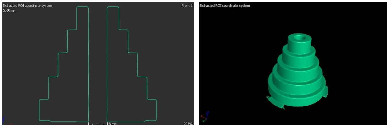
Figure 4.36. Meshed CT images of step cylinder of aluminum step cylinder
