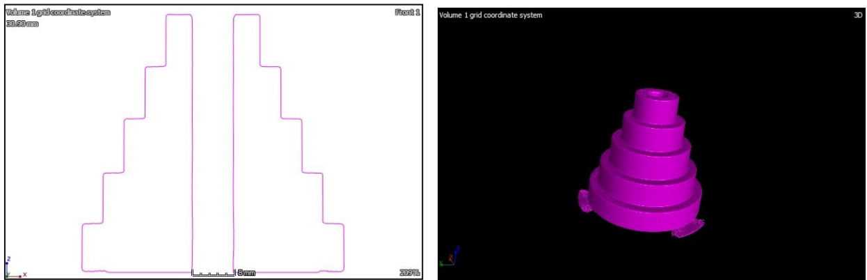
Figure 4.35. Meshed CT images of scan8 parameter set of plexiglass step cylinder
