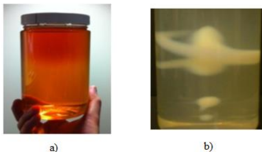
Fig. 3. Examples of various gel dosimeters: a) Fricke gel dosimeter irradiated with 12 MeV electron beams demonstrate color change; b) polymer gel dosimeter irradiated using intensity-modulated radiation therapy [1].
