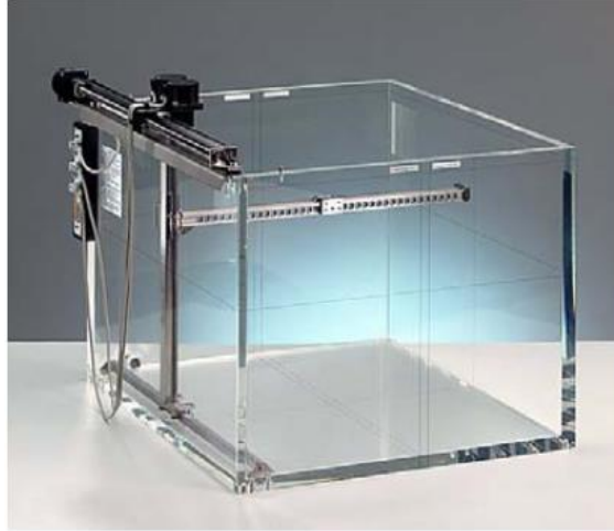
Fig. 8. Small water phantom for absolute dosimetry [33]
