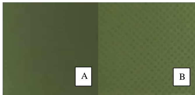
Fig 24. 2D GafChromic films EBT2 irradiated between the standard CT PMMA head phantom and the 3D printed polylactic acid plastic (PLA) bolus. A – irradiated GafChromic film under the 100 % infill ratio 3D printed PLA bolus. B – irradiated GafChromic film under the 90 % infill ratio 3D printed PLA bolus [49]
