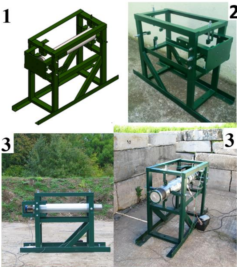
Fig. 3.3. Structure of the rocket motor test stand
