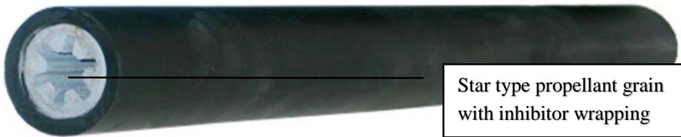
Fig. 2.3.13. Produced propellant grain. Refer to Fig. 3.2 item 4
