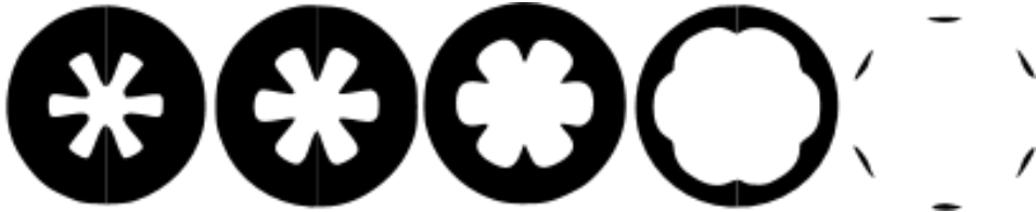
Fig. 2.3.2. Evolution of the propellant grain due to interface tracking [87]
