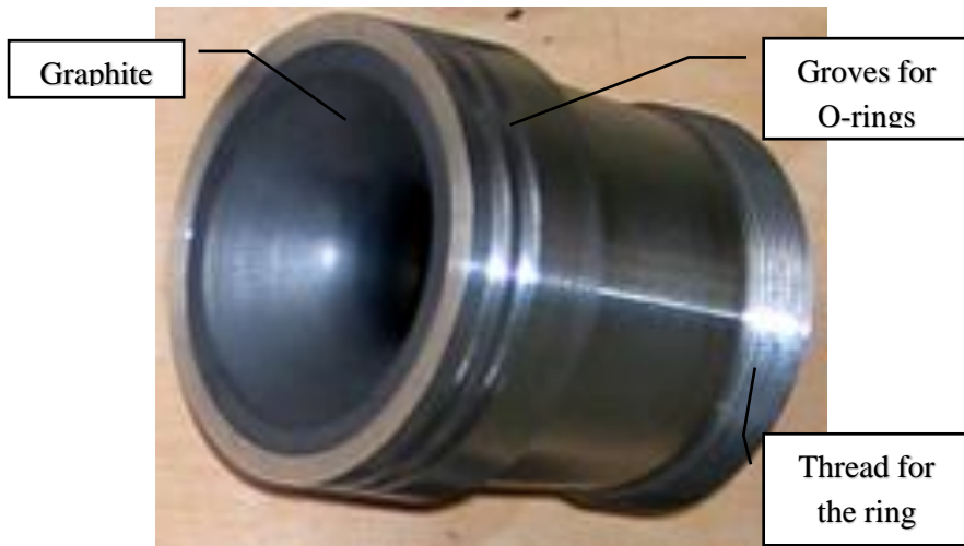
Fig. 2.3.11. Nozzle part which was made for production. Refer to Fig. 3.2 item 3
