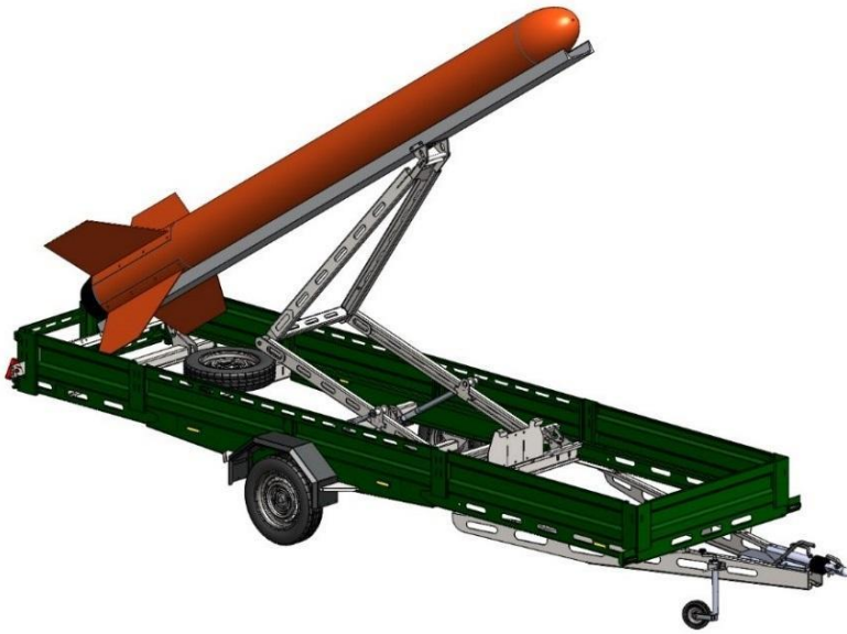
Fig. 1.4.1. RT-400 Aerial target system with RM-12K solid-propellant rocket motor
