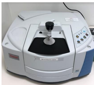
Figure 2.7.1. ThermoScientific Nicolet iS10 FTIR
