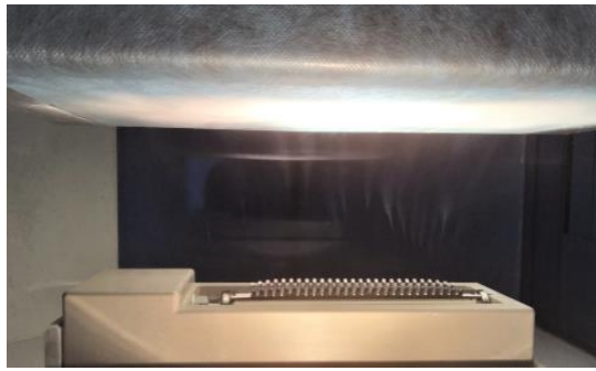
Figure 2.5.3. Electrospinning process in Nanospider
