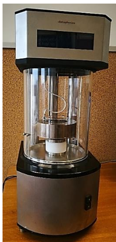
Figure 23. Dynamic contact angle measuring devices and tensiometer DCAT 21 (DataPhysics Instruments GmbH, Germany)
