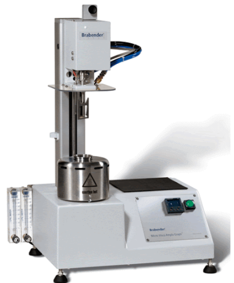
1.10 pav. Klamos matavimo prietaisai Micro Visco-Amylo-Graph® (Brabender, Germany) [15]
