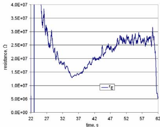
Fig. 8. The alternation of the identified inner resistance of the supply during the process
