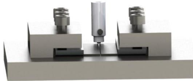
Fig. 2 Experimental scheme. The tool welds two ABS plastic plates together with set friction stir welding parameters. Then welded plates are left to cool
