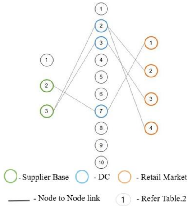
Fig. 16. Optimum network design of a stochastic model with maximum scenario cost with N=2
