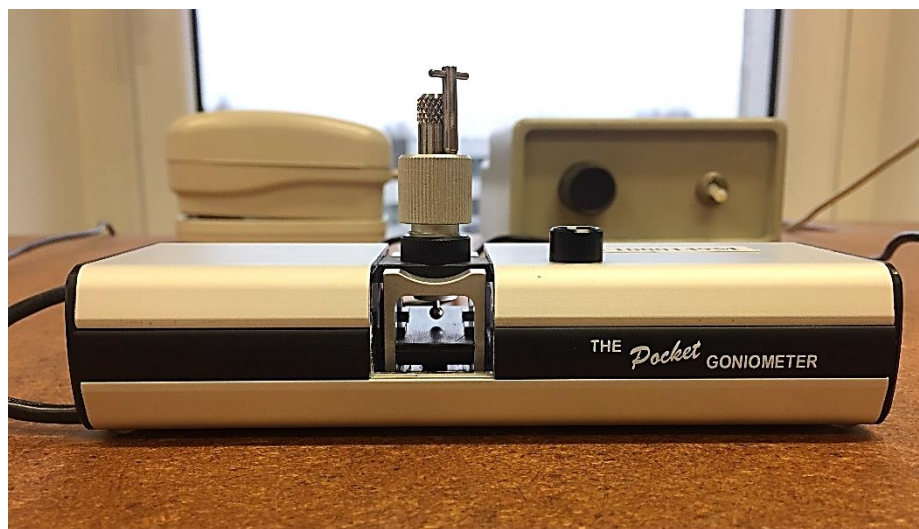
Fig. 8. Pocket goniometer 3 (PG3) device for contact angle measurements
