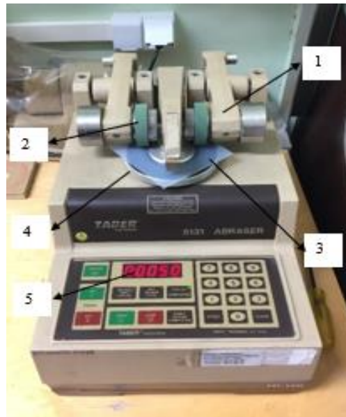
Fig. 9. Experimental setup of surface abrasion treatment: 1- mechanical arm; 2- abrader wheels; 3- PA6 specimen; 4- rotating disc; 5- digital meter
