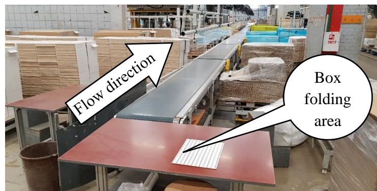
Fig. 11. Manual box folding area, SC “Freda” packaging line
