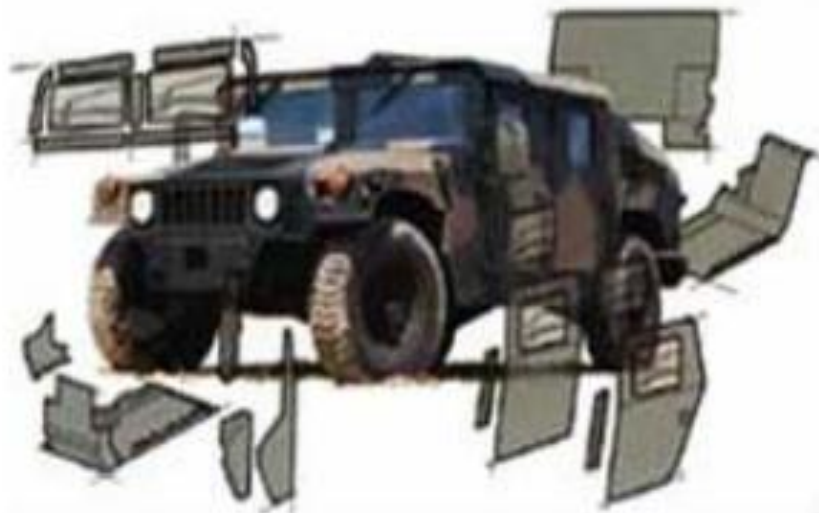
10 pav. Homogeniniai šarvai ant visureigio HMMWV [21]
