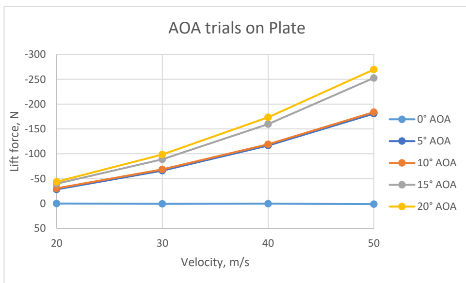
Fig. 49. Lift force for angle of attack trials on plate type profile
