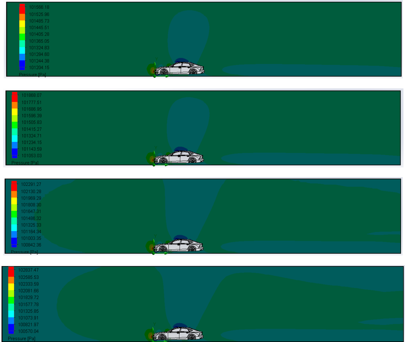
Fig. 22. Pressure distribution for case 1 at different velocities; 20 m/s, 30 m/s, 40 m/s and 50 m/s (from top to bottom)
