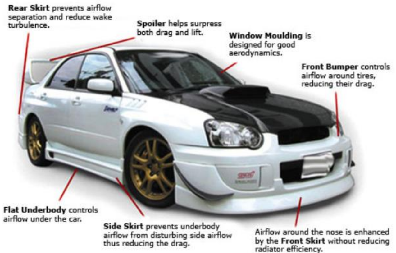
Fig. 2. Aerodynamic components of a car [26]
