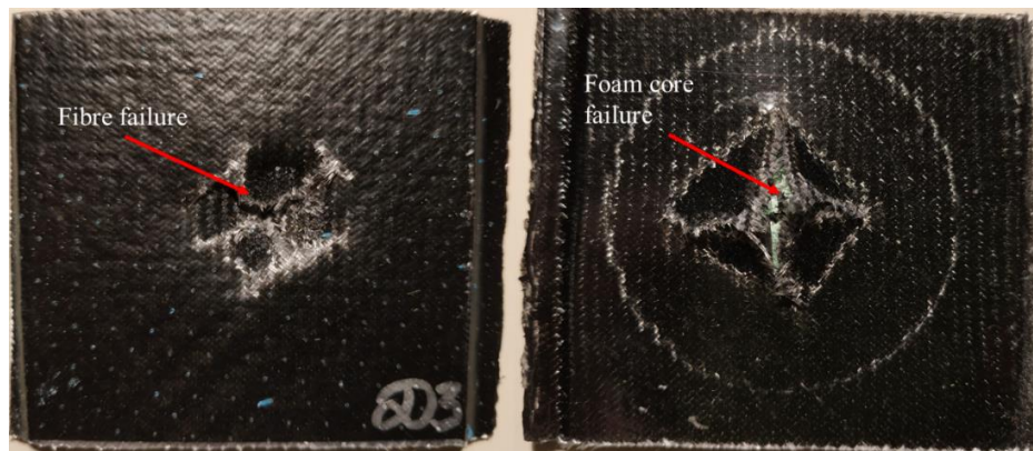
Fig. 23. Specimen with 0.75wt.% of CNTs matrix after the puncture
