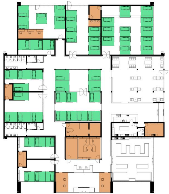
Figure 93. Diagram of an adaptation of the daycare to a medical center.
