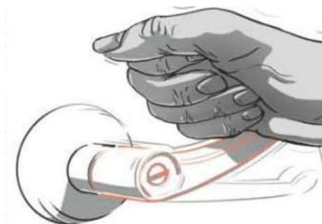
Figure 8. Door lever can be operated with closed fist or elbow, unlike door knobs (Michael A. Capuano & Camila Sainz De La Peña, 2015).
