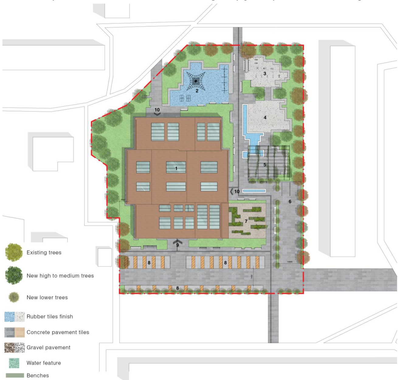
Figure 85. Site plan (not to scale): 1. Daycare center; 2. Outdoor playground; 3. Outdoor sports zone; 4. Outdoor area for other activities; 5. Outdoor lounge area; 6. Service car park; 7. Outdoor garden; 8. Parking area for visitors; 9. Main entrance; 10. Secondary entrance.
