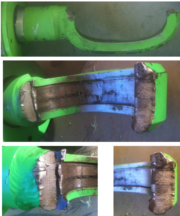
Fig. 1 Photos of the broken eye of the hydraulic cylinder rod
