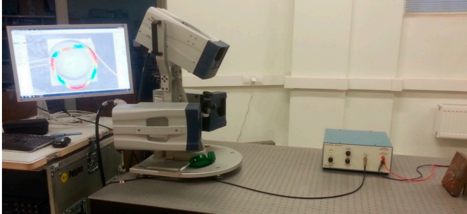
Figure 9. Experimental setup with Polytec Laser Doppler Scanner. 1 - PSV-500 3D scanning Head of the vibrometer; 2 – PSV-500 3D scanning vibrometer and PC; 3 – optical table; 4 – amplifier EPA-100 (PiezoSystems Inc., USA); 5 – Steel plate with the mounted piezoelectric ring. The piezoelectric ring is mounted on a metal plate and fixed with double-sided adhesive tape.
