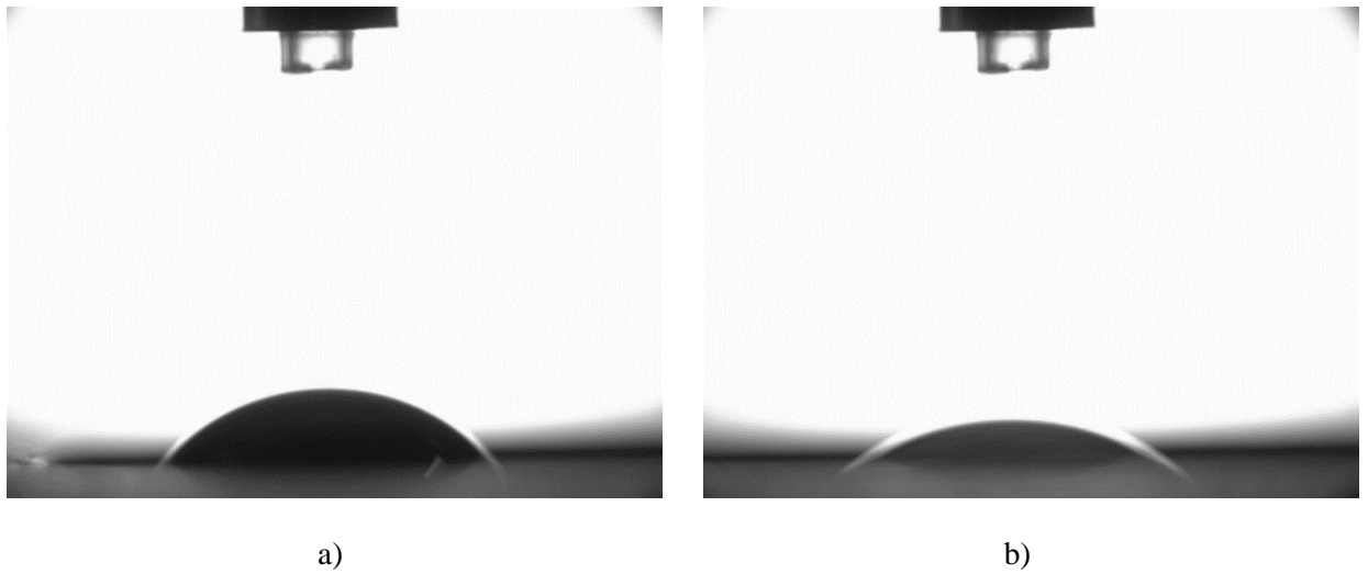
Fig. 11. View of droplets on HDPE A30 material a) printing side, b) non-printing side
