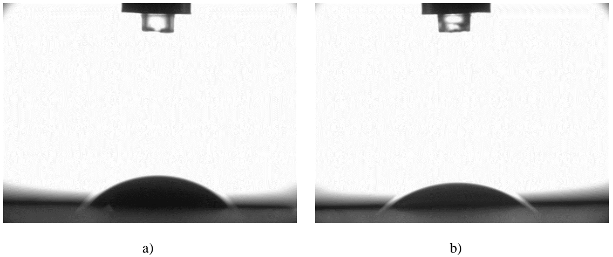
Fig. 13. View of droplets on HDPE A50 of material a) printing side, b) non-printing side
