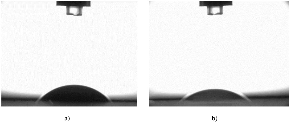
Fig. 7. View of droplets on HDPE material a) printing side, b) non-printing side
