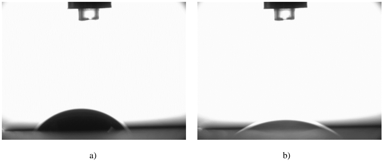
Fig. 15. View of droplets on RHDPE material a) printing side, b) non-printing side
