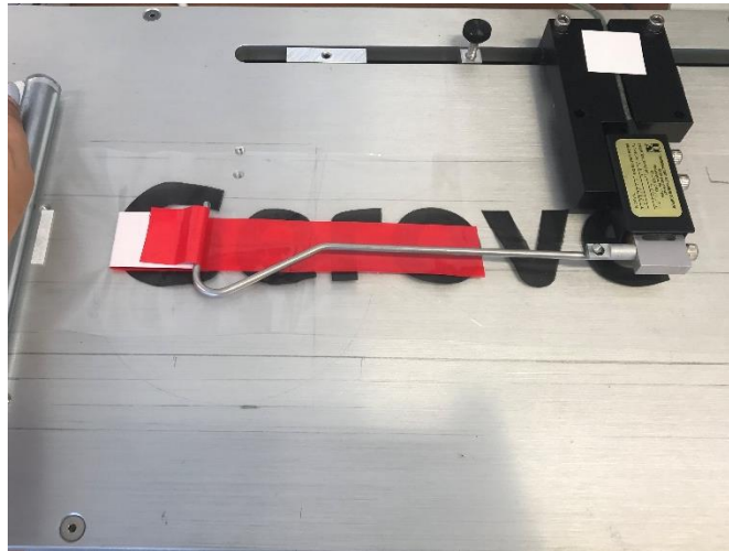
Fig. 25. Ink adhesion test with measured force
