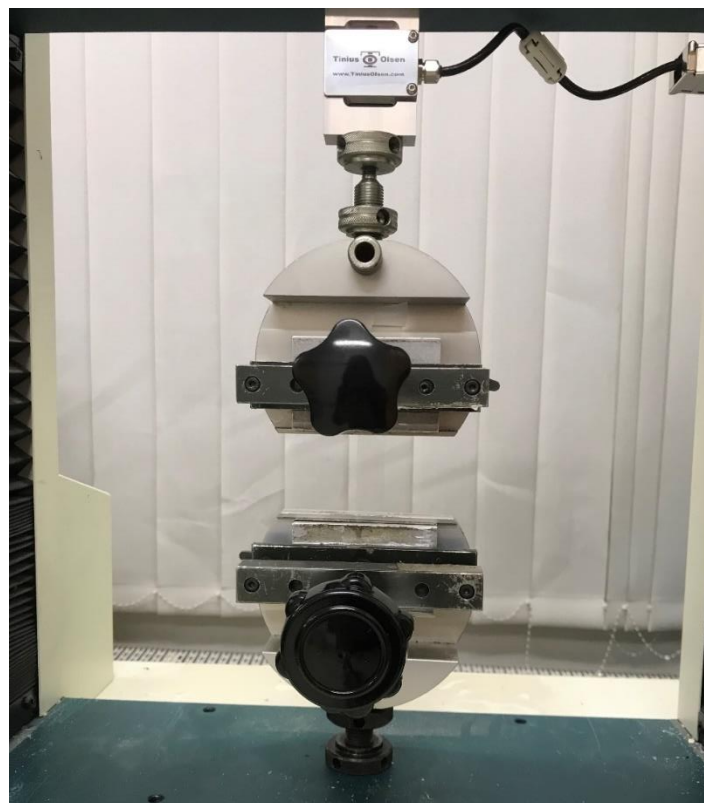
Fig. 6. View of material fixed between clamps for tension test
