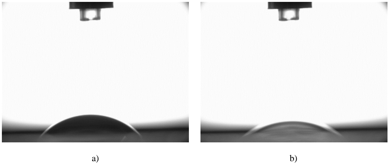
Fig. 9. View of droplets on HDPE A15 material a) printing side, b) non-printing side
