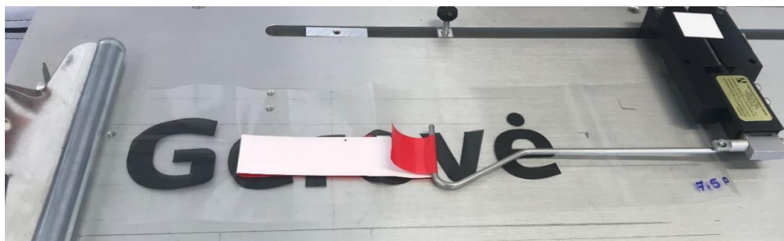
Fig. 26. Ink adhesion test with measured force
