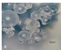
Microcapsules with Allium cepa essential oil core in different shells: a - polystyrene, b - ethylcellulose
