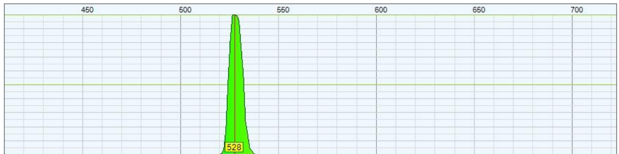
Fig. 37 The spectrum of green laser with a peak at 528 nm obtained after calibration.
