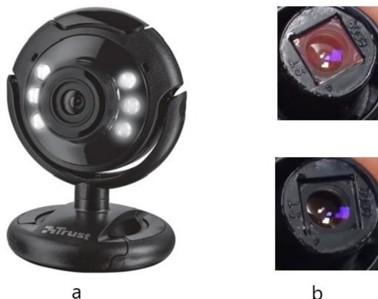
Fig. 25 a) Trust web camera used in the spectrometer; b) Removal of IR filter
