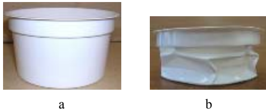
Fig. 7 External view before (a) and after (b) compression of I type (6069/L) of PS package
