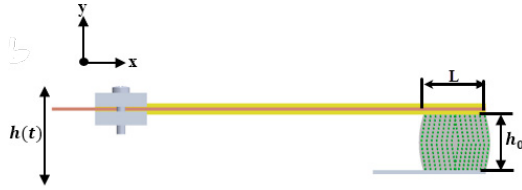
Fig. 6 Squeezed ERF film between a fixed bottom and vibrating electrode
