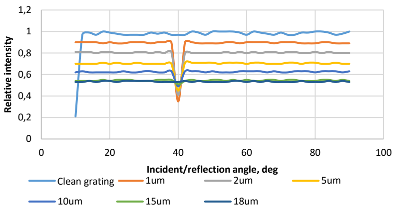
Figure 16. Readout results of plasmonic sensors with different thicknesses of the VIPET dosimetric gel layer
