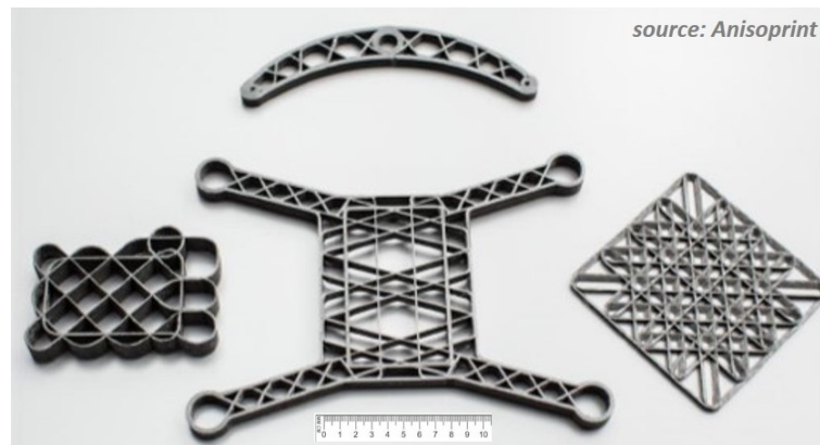
Figure 7. Three-dimensionally printed CFRP composite structural parts based on bi-matrix TS-TP FFF technology.
