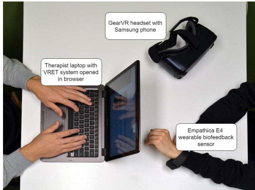
Figure 1. Key components of the virtual reality exposure therapy (VRET) system.
