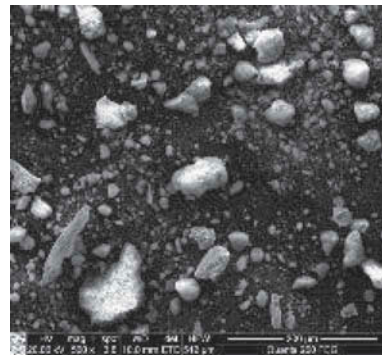
Figure 8. The SEM images of oxidation products on surface of weather-resistant steel samples.
