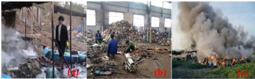
Figure. 1.1.5. Environmental risks of primitive WPCB recycling techniques: (a) precious metals recovery by acid leaching; (b) unprotected WPCB dismantling; (c) open burning of WPCBs (Huang et al. , 2009)
