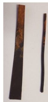
Figure 1. Black deposit on the surface of copper, which was formed during copper dissolution in concentrated sulfuric acid
