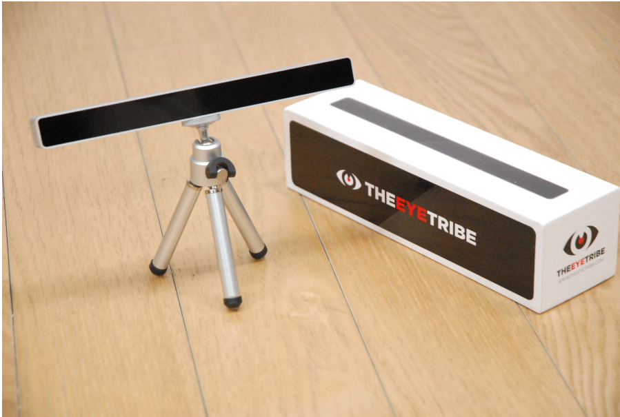
Figure 5.2. The eye tracking device Eye Tribe.
