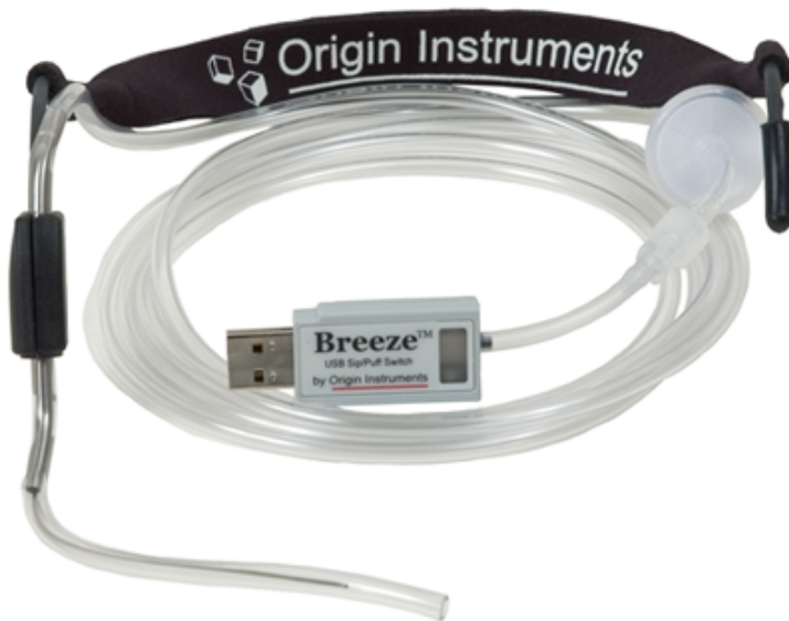
Figure 5.3. The Sip/Puff device from Origin Instruments Sip/Puff Breeze.
