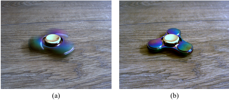
Figure 4.11. The effects of shutter speed on moving objects. (a) long shutter speed image with motion blur, (b) short shutter speed image with no blur.
