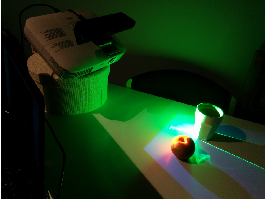
Figure 4.2. Example projection mapping user interface scene setup. The camera-projector system is placed in front of the tabletop scene with objects highlighted in different colors.
