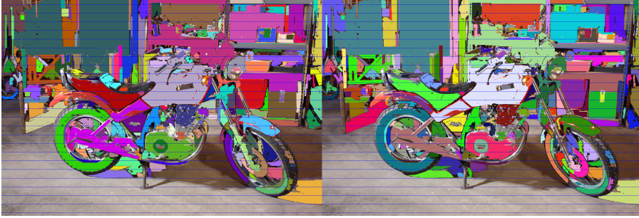
Figure 4.14. Stereo image pair with detected MSER colored randomly. The blue lines show epipolar image lines every 20 pixels.
