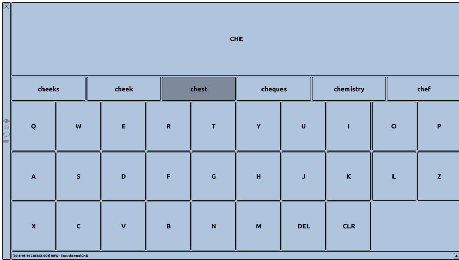
Figure 3.7. TextInput screen example. The screen is divided into the entered text area (top), the predictions area (middle) and the keyboard keys (bottom). There are additional status bars at the bottom and left side of the screen.
