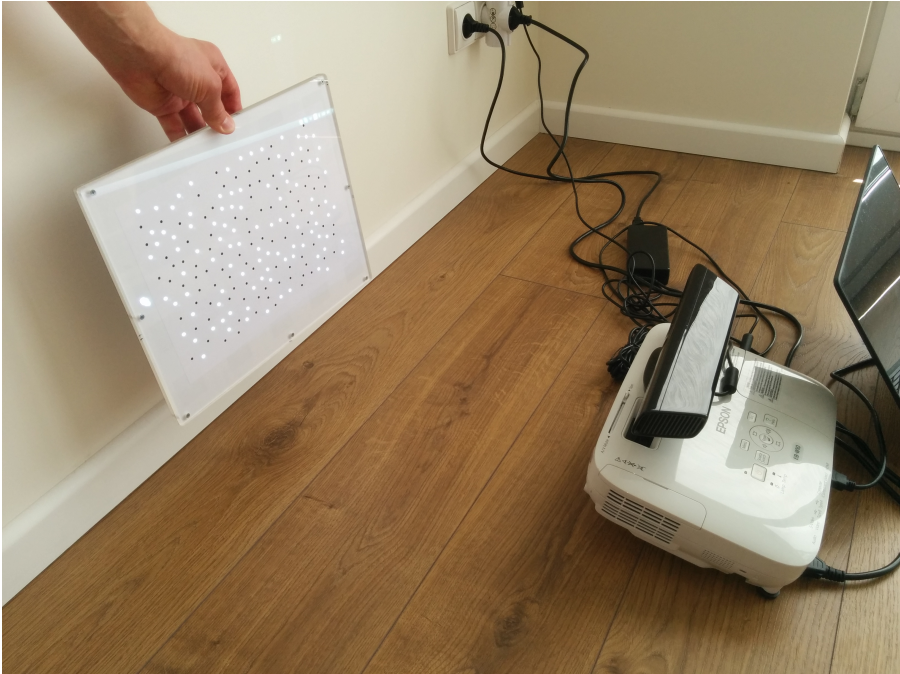
Figure 4.4. Camera-projector system calibration by using a board with a circular black dot pattern. White dots are created by using a projector.
