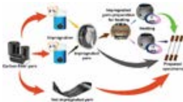
Fig. 1 Procedure of carbon fibre modification
