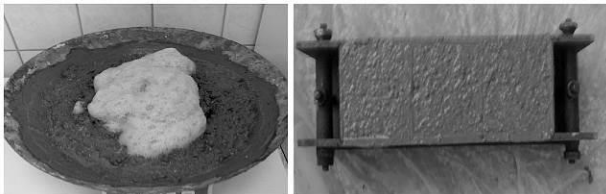
Figure 1. Mmixing foam with cement mortar and Moulded concrete
